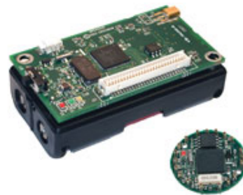
Figure 1. Two Berkeley Motes, the Mica2 (top left) and the Mica2Dot(bottom right)
